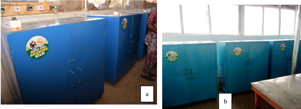
Figure 2: NSPRI Smoking Kilns in the Fish Processing Centres. a. Electricity powered type, b. Charcoal powered type
