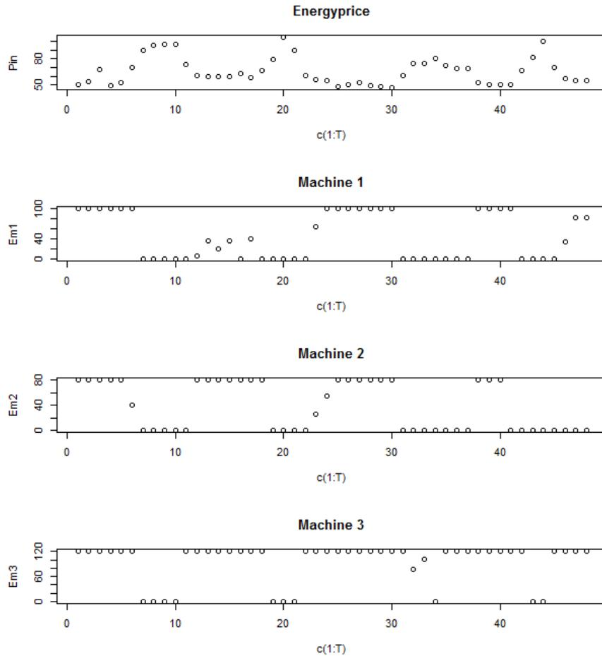
Figure 1: The effect of fluctuating energy prices in an energy efficient production planning
