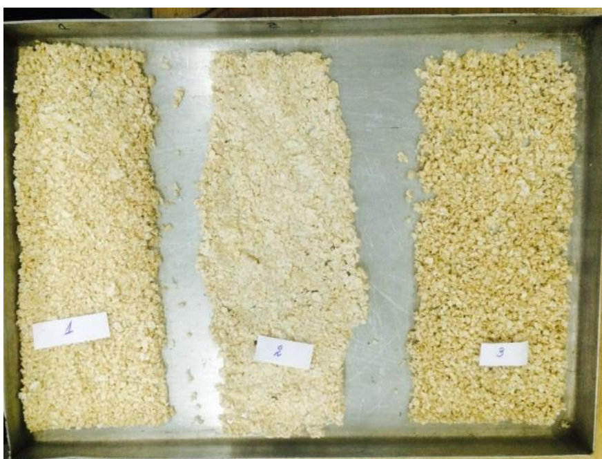
Figure 1. Hydrolysates after vacuum freeze drying: 1 - hydrolysate obtained by enzymatic hydrolysis, 2 - hydrolysate obtained by chemical hydrolysis (with acids and alkalis), 3 - hydrolysate obtained by the method of natural structuring (hydrothermal method)
