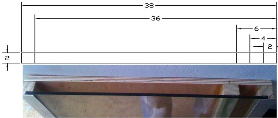
Figure 1: Schematic drawings of the front view (upper photo plate) and top view (bottom photo plate) of the rhizobox used with measurements in cm
