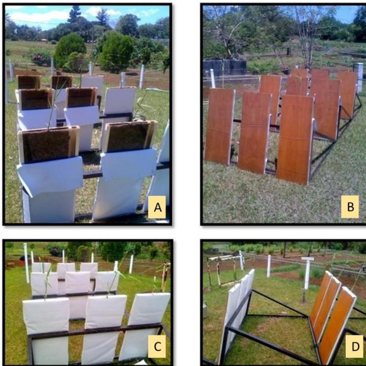
Figure 2: Rhizoboxes showing A. glass pane uncovered; B. front wooden side; C. glass side covered with tarpaulin; and D. side view held by a metal frame
