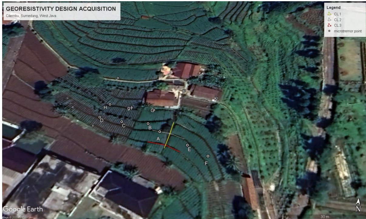
Figure 2: microtremor measurement stations (A, B, C, D, E, F, G, g1, H, I, J, K), and ERT design acquisition (CL 2, CL 2, CL 3)
