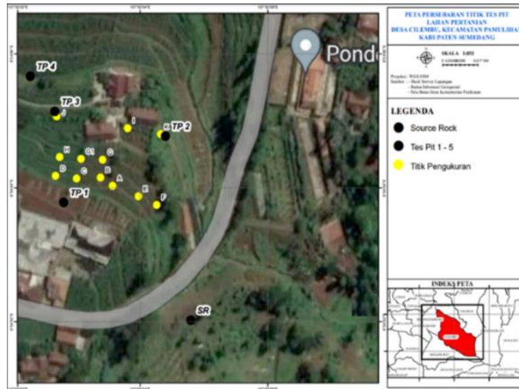
Figure 3: test pit location (TP1, TP2, TP3, TP4), and source rock locations (SR).
