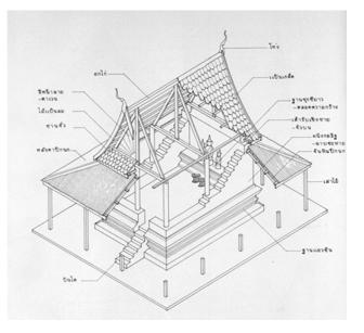
Figure 7: The structural elements of Sim.
