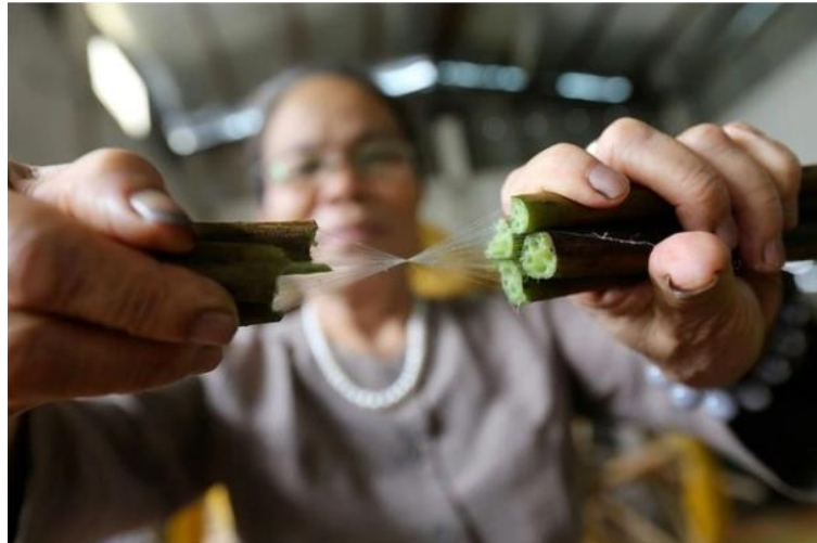
Figure 60: Cutting on the lotus stem must be just right—if it's too deep, the silk fibers inside will break; if it's too shallow, the stem won't twist to extract the fibers, source:[39]
