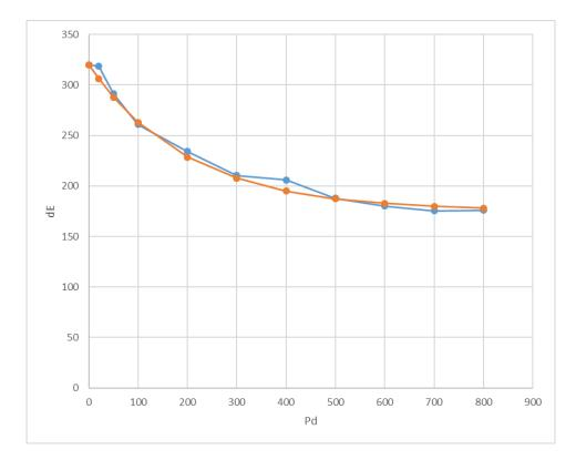
Figure 2: Bidirectional demand charge (x-axis) and maximal difference between energy consumption and energy generation (y-axis) with model results (blue) and regression (orange)
