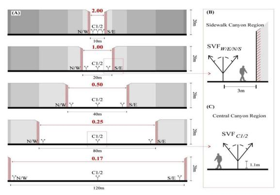
Figure 2: Layout of the determined Sky-View-Factors (SVF) within the four stipulated Aspect Ratios (AR) (Nouri, A. S., Costa, J. P., & Matzarakis, A. 2017)
