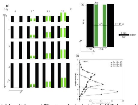
Figure 1: Schematic diagrams of different scenarios showing (a) vertical (XZ) view trees of different ART in street canyon of different ARB, (b) the XY view with the location of Vertical Cut for Analysis which was taken at the middle of the street canyon (Morakinyo et al 2016).
