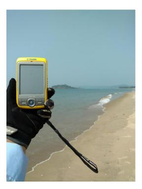
Figure 16: shows Trimble GPS which was used for Shoreline Tracking
