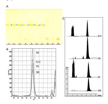
Figure 3: (A) TLC image of standard Sibutramine (track 1), adulterated slimming formulations (tracks 2–7: S2, S6, S7, S9, S10 and S19) and Sibutramine-free samples (tracks 8–10: S14, S15 and S16), (B) TLC
