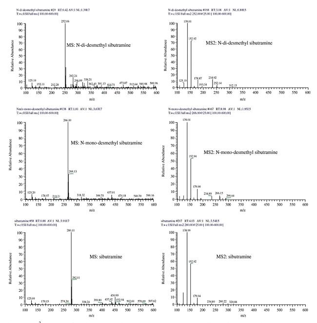
Figure 7: MS<sup>2</sup> spectrum of N-di-desmethyl sibutramine, N-mono-desmethyl sibutramine, sibutramine. The mass spectrometer used was a Finnigan LCQ Advantage MAX (Thermo, USA). ESI+; sheath gas flow rate: 40 arb;
