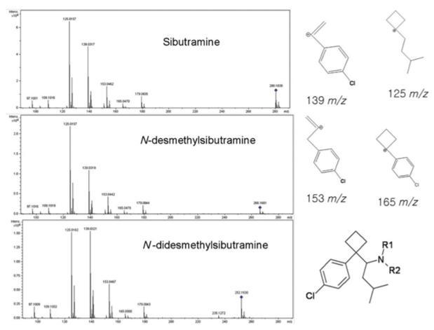
Figure 9: Mass fragmentation pattern and fragment compounds of the compound Sibutramine and its analogues. (Roh *et al.*, 2011)
