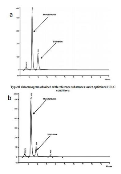
Figure 6: (a) Typical chromatogram obtained with reference substances under optimized HPLC conditions and (b) the chromatogram obtained with capsule content of an adulterated for the herbal supplement (CS) (Ancuceanu, Dinu and Arama, 2013)
