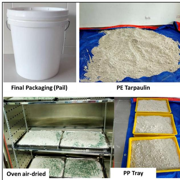
Figure 2: Powder formulated M103 dried using different techniques
