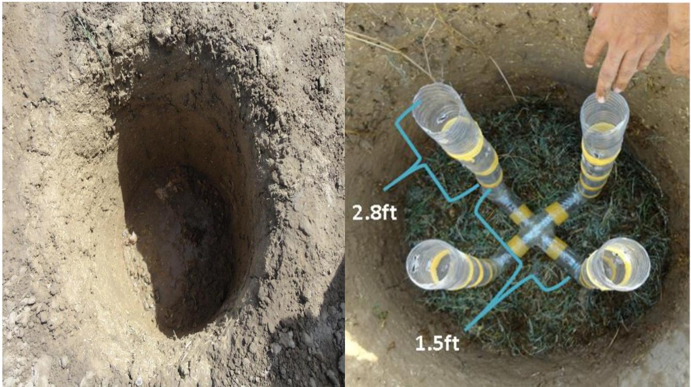
*Fig. 3. (A) Soil pit. (B). Semi aerobic soil pit with perforated pipes*
